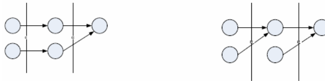
Figure-5 Step 3(A): generating the two connections for the shape (2,2,1) – the two topologically distinct trees formed by connecting each LUT output in a layer to a LUT input in the next layer.
