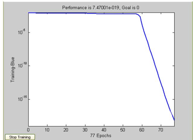
**FIG 8: PERFORMANCE OF A FFBP-NN WITH ORIGINAL DATA HAVING 60 DIMENSIONS**
