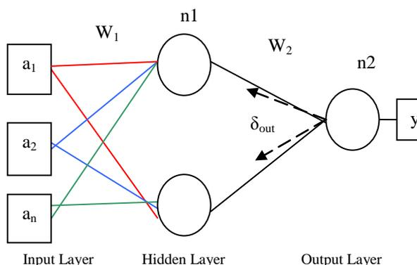
Figure 2. Simple Back Propagation Neural Network
